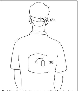
**Fig. 1** Illustration of tri-axial accelerometers affixed  ${\bf A}$  to a headband and  ${\bf B}$  to the participant's back
