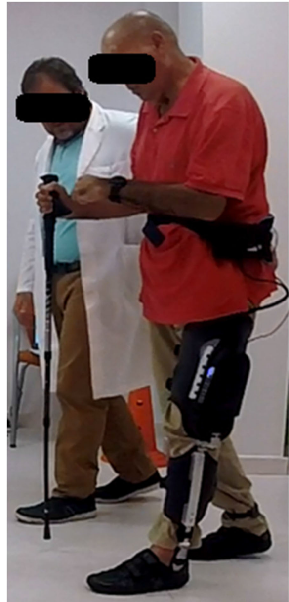
Fig. 8 Participant using the MAK exoskeleton during a trial
