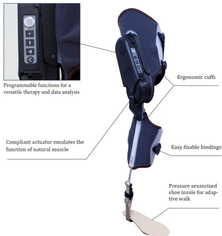
Fig. 1 Marsi Active Knee (MAK) exoskeleton, by Marsi Bionics
