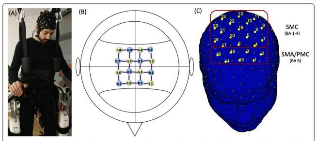
**Fig. 1** Montage and Setup. **a** Participant during robot-assisted walking (RAW), with functional near-infrared spectroscopy (fNIRS) montage. **b** fNIRS montage; S = Sources; D = Detectors **c** Classification of regions of interest (ROI): supplementary motor area/premotor cortex (SMA/PMC) and sensorimotor cortex (SMC)
