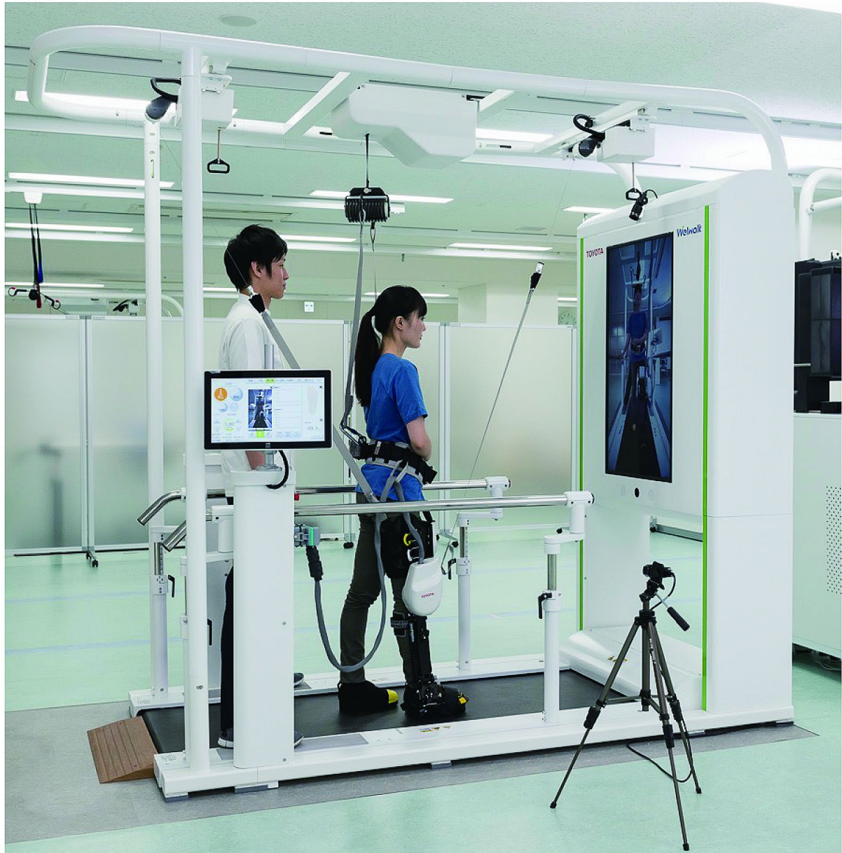
Fig. 1 Overview of the Welwalk WW-1000. The Welwalk WW-1000 is composed of a knee-ankle-foot orthosis-type robotic leg, a low-floor treadmill, a safety-suspending device (which can be used as a body weight support device), a robot weight-support device, a monitor for patient use, and a control panel. The robotic leg is equipped with a motor in the knee joint and a load sensor on the sole, which is used to calculate the gait cycle. The patient wore the robotic leg only on the paralyzed lower limb. All robot operations were controlled using a control panel. In most patients with hemiparetic stroke, gait training can be performed by a single therapist
