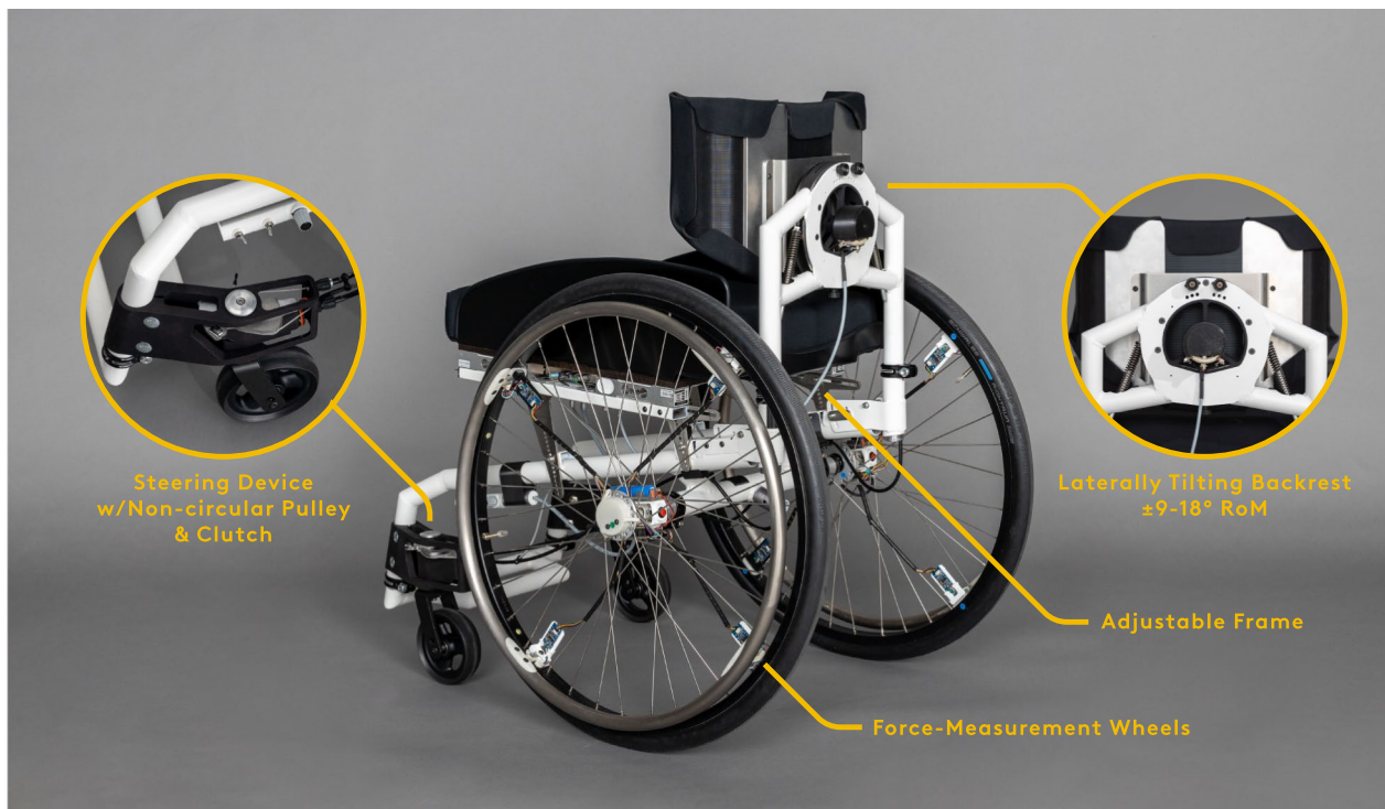
Fig. 2 Study prototype wheelchair with a steering-by-leaning system: If engaged, a laterally tiltable backrest acts as a steering wheel that controls the orientation of the front wheels and, therefore, the direction of wheelchair movement
