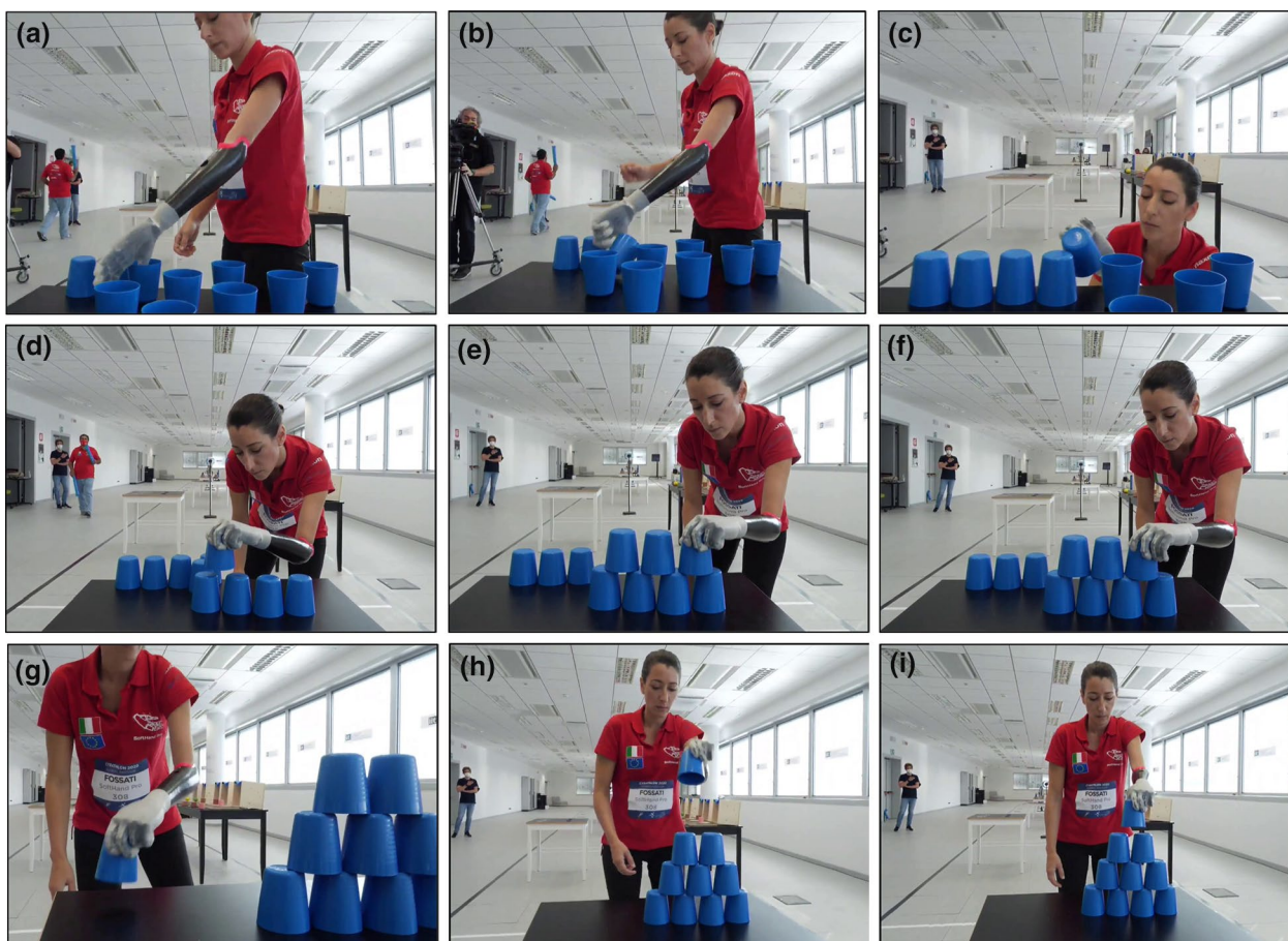
Fig. 14 Photo-sequences of the stacking Task (#6, Cybathlon 2020). a–c Show the turning glasses phase. d–f Present the building of the pyramid, paying attention to the releasing due to the lack of sensory feedback and the instability of the pyramid. g–i Show the last glass positioning, which is the most difficult one and, because of the height of the Pilot B, it requires an unnatural position of the shoulder to release the glass parallel to floor
