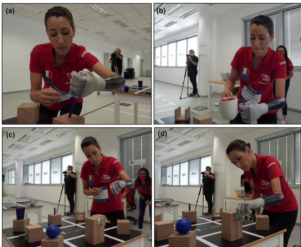
Fig. 11 Different grasping patterns corresponding to the object shape and requirements: a a pen, b a mug full of wooden-balls and c, d are different instants of the grasping and moving of a key
