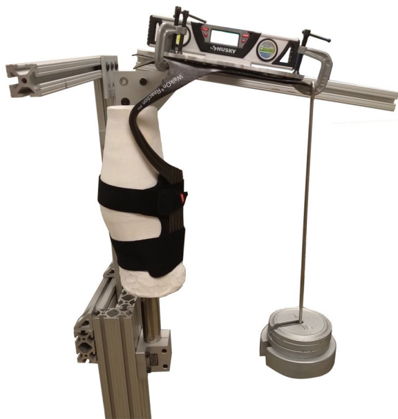
Fig. 2 Setup for hanging weight method. In this approach, an AFO is strapped to a surrogate shank and the footplate is clamped to a backing plate. Weights are hung from the AFO toe and the angle of deflection is measured with an inclinometer. Torque is computed from the applied load and the moment arm measured to the center of the surrogate shank
