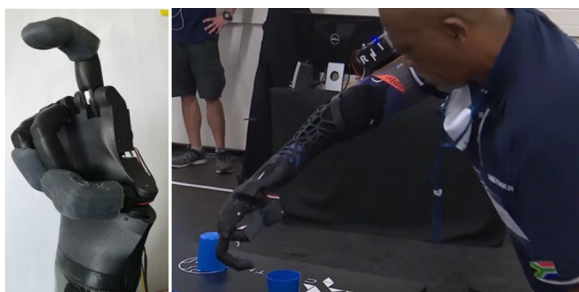
Fig. 16 Pilot demonstrating the half grip using the Touch Hand 4.5
