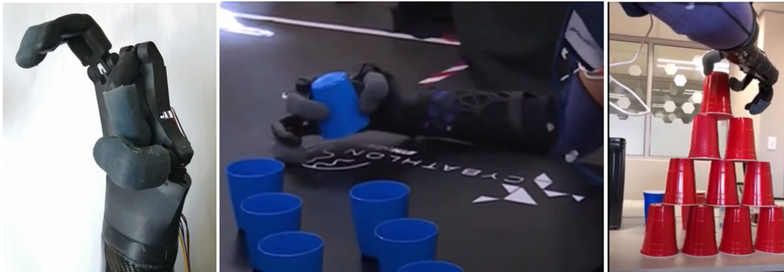
Fig. 14 Touch Hand 4.5 demonstrating the pinch grip
