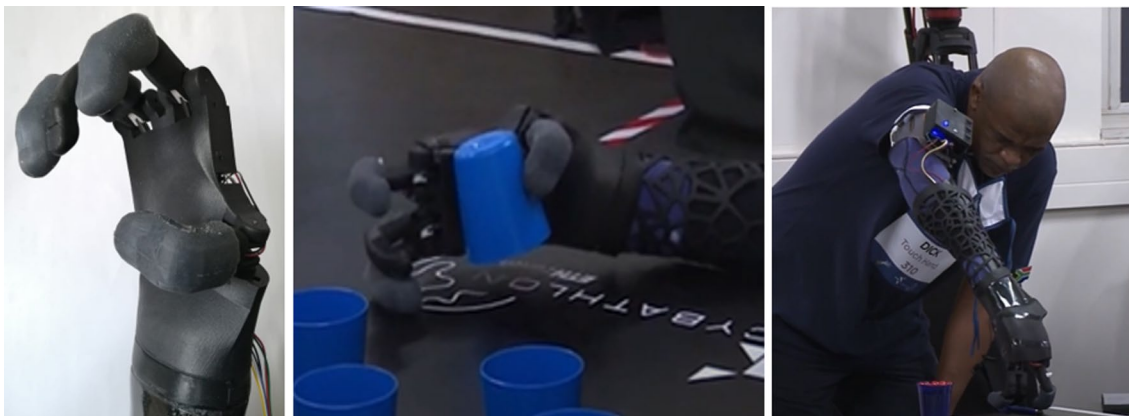
Fig. 17 Pilot using the thumb grip to complete different tasks in the Cybathlon 2020 event
