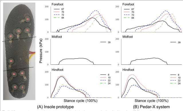
Fig. 7 A Representative measured pressure patterns using the insole prototype developed in this study and **B** Corresponding pressure patterns using a Pedar-X system during stance phase
