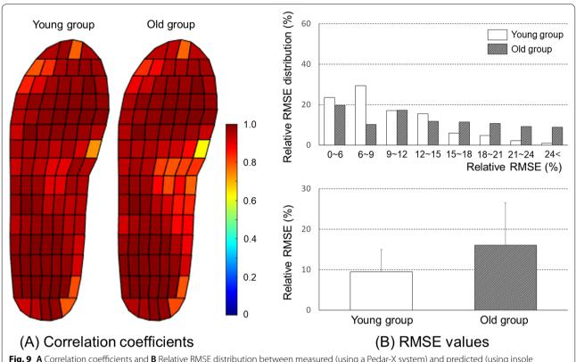
Fig. 9 A Correlation coefficients and B Relative RMSE distribution between measured (using a Pedar-X system) and predicted (using insole prototype and LSTM model proposed in this study) pressure patterns
