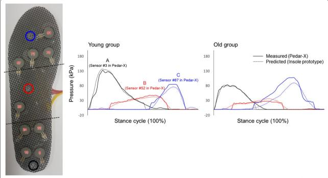
**Fig. 8** Representative measured (using a Pedar-X system) and predicted (using the proposed LSTM model from nine FSR sensor signals of the insole prototype as model input) pressure patterns during stance phase
