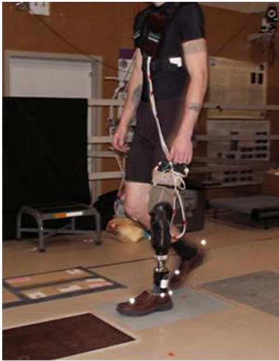
Figure 2 Example of system setup and walking condition. The EMG gain box is shown strapped to the subject's chest. After signal gain and band-pass filtering, the EMG signals were transmitted via FM radio frequency to a receiver near the analog breakout box and A/D board.
