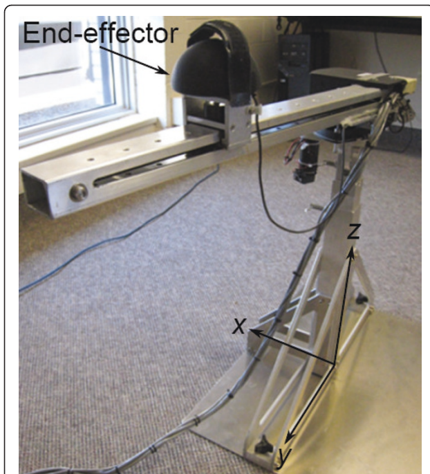
Figure 3 Actual robotic rehabilitation device. The robotic rehabilitation device features a non-restraining platform and allows the reaching exercise to be performed in 3D space.
