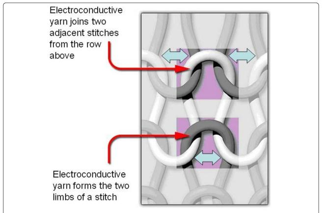
**Figure 1 Structure of the resistive strain sensor**. The individual stitches which make up the knitted resistive strain sensor. The electroconductive yarn is shown in white and arrows mark the regions where electrical contact is made as the base structure relaxes after stretching.
