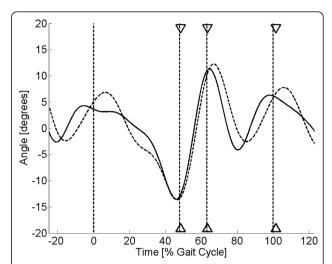
**Figure 5 Sensor output (sock-only condition) for subject 1.** Plot of sensor output (solid line) and scaled kinematic signal (dashed line) against time for a single walking trial from subject 1 (sock-only condition). The three sets of triangles show the estimated times of heel lift, toe off and heel strike with the vertical dashed lines showing the true values.
