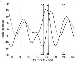
**Figure 8 Sensor output (shod condition) for subject 9.** Plot of sensor output (solid line) and scaled kinematic signal (dashed line) against time for a single walking trial from subject 9 (sock-only condition). The three sets of triangles show the estimated times of heel lift, toe off and heel strike with the vertical dashed lines showing the true values.
