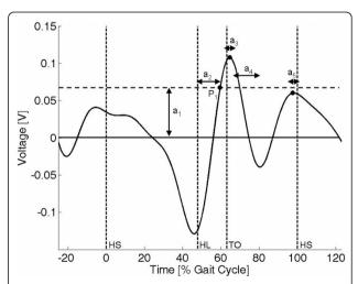
**Figure 9 The event detection algorithm.** Plot to illustrate the five parameters used in the event detection algorithm.
