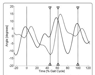
**Figure 6 Sensor output (sock-only condition) for subject 20**. Plot of sensor output (solid line) and scaled kinematic signal (dashed line) against time for a single walking trial from subject 20 (sock-only condition). The three sets of triangles show the estimated times of heel lift, toe off and heel strike with the vertical dashed lines showing the true values.
