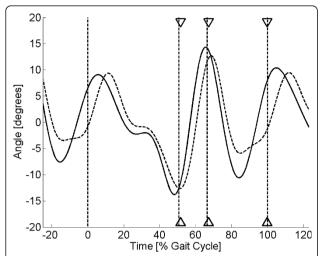
**Figure 7 Sensor output (shod condition) for subject 8.** Plot of sensor output (solid line) and scaled kinematic signal (dashed line) against time for a single walking trial from subject 8 (shod condition). The three sets of triangles show the estimated times of heel lift, toe off and heel strike with the vertical dashed lines showing the true values.
