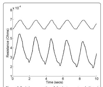
**Figure 2** Resistive properties of the instrument sock. Plot of resistance (solid line) against time showing how the knitted sensor responds to a periodically applied strain (dotted line). This data shows a gradual drift in the baseline resistance after several successive stretches.
