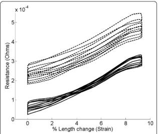
**Figure 3** Resistive properties of the instrument sock. Plot of resistance against length change over several stretch-relaxation cycles (dotted line) and the same data after high pass filtering of the resistance data (solid line).
