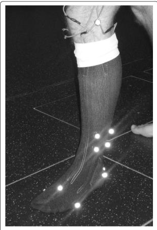
**Figure 4 Experimental set up**. Image of the instrumented sock with the kinematic markers used for data collection during the sock-only walking trials.
