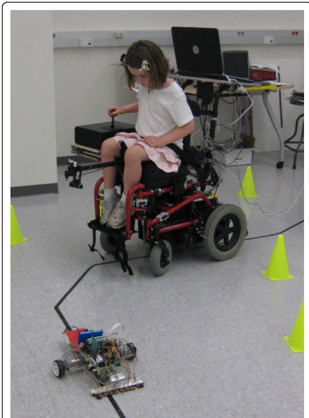
Figure 1 ROLY -RObot-assisted Learning for Young drivers. We developed a robotic wheelchair trainer that steers itself along a course marked by a line on the floor using computer vision, haptically guiding the child's hand in appropriate steering motions using a force feedback joystick. The child is instructed to follow the line with a spot of light from a laser pointer mounted on the chair, creating the smallest amount of error possible. To motivate the children during training, we programmed a small mobile robot to follow the same black line, and requested the child to try to catch it in a game of "robot tag".
