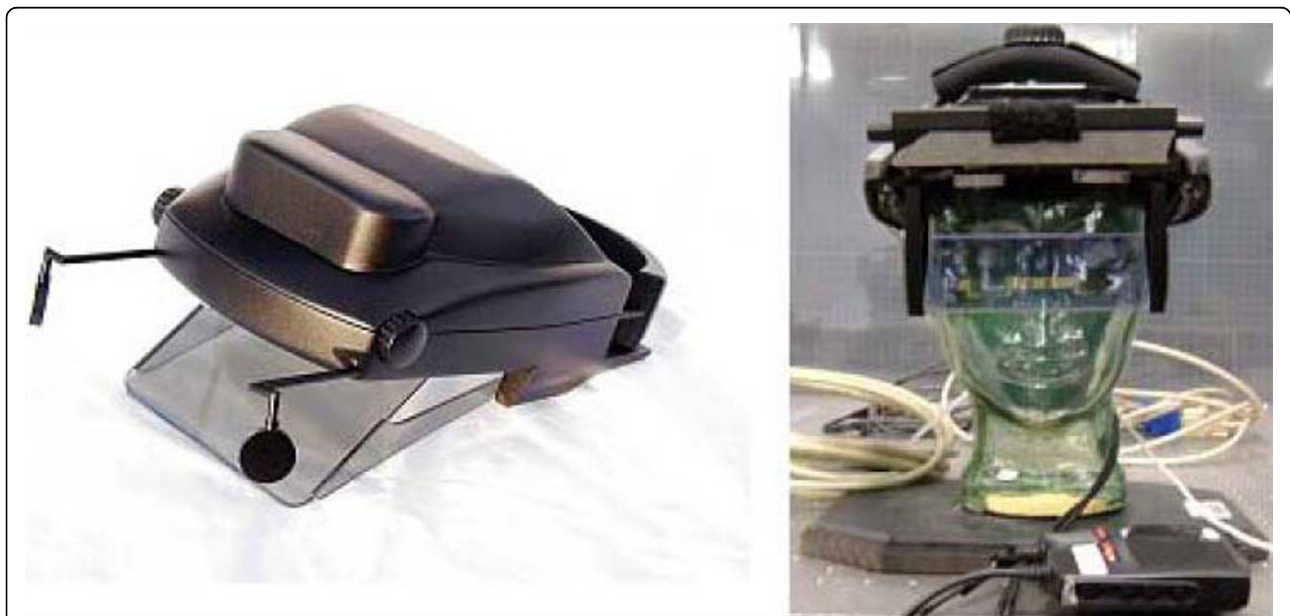
Figure 3 Optical See-through HWD prototypes. First (left) and second (right) generation prototype head-mounted projection displays developed in the University of Central Florida.
