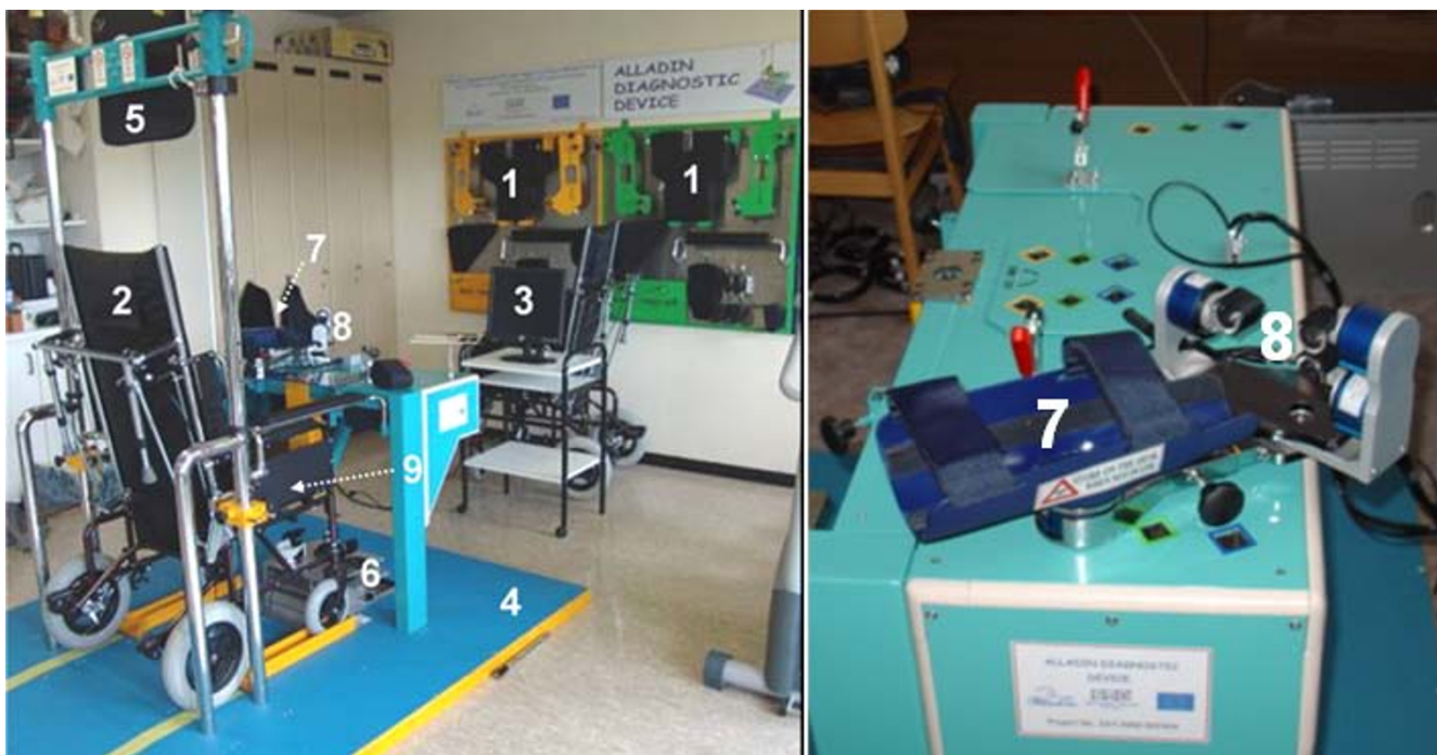
Figure 2 The components of the platform: 1) Accessory storage board, 2) Transit lying wheelchair, 3) Monitor for the patient, 4) Podium, 5) Trunk Device, 6) Foot Device, 7) Arm Device, 8) Finger Device, 9) Seat Device.
