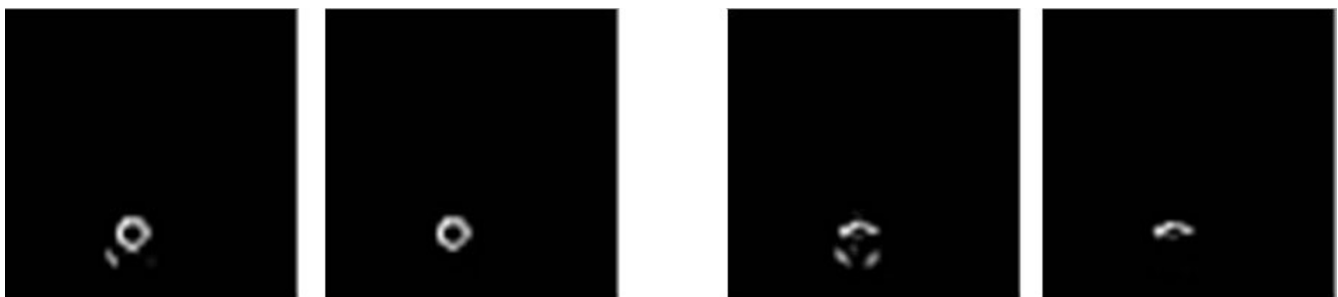
Figure 6 The mouth detection results. (a) edge detection results, (b) noise removed results.
