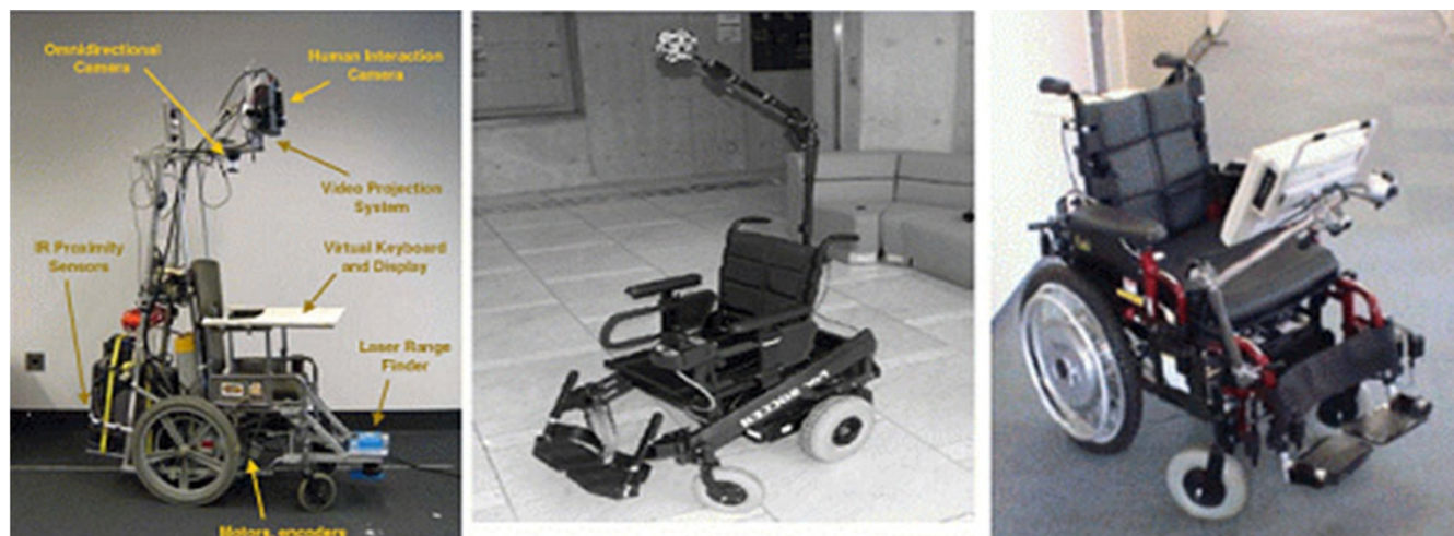
Figure 1 Intelligent Wheelchairs (IW). (a) GRASP Laboratory Smart Chair [6], (b) Wheelchair of Yutaka et. al [3], (c) Nav Chair [14].
