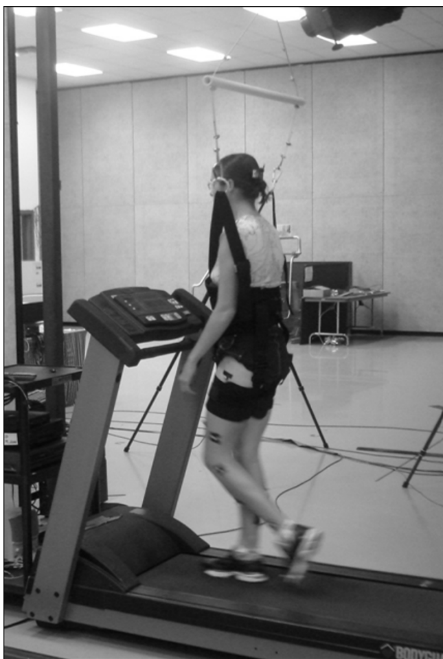
Figure 1 A subject walking at 1 g while being suspended by the Body Weight Support System.
