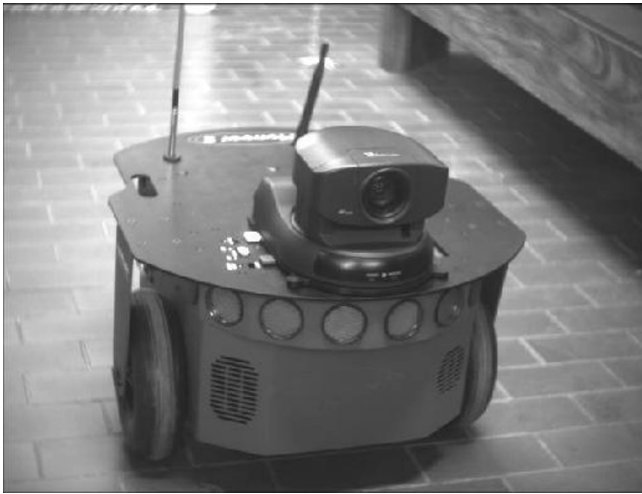
Figure 11 Pioneer 2-DX robot operated through EEG signals.
