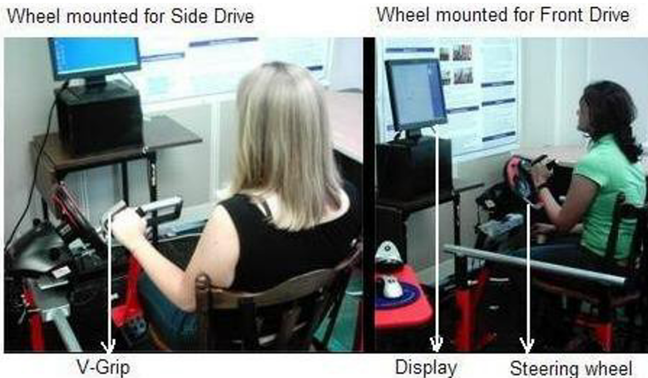
Figure 3 TheraDrive System for home-based rehabilitation. This figure shows the driving wheels mounted in front and side configurations with the subject holding onto a v-gripper.
