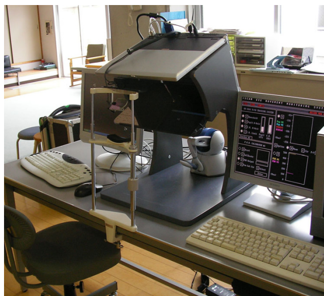
Figure 1 System. From left to right: virtual world monitoring, immersive workspace with eye-tracking device and a Phantom Omni haptics device, eye-tracking computer.
