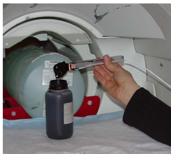
Figure 6 Simple device that was used to test the MR compatibility of ERFs.
