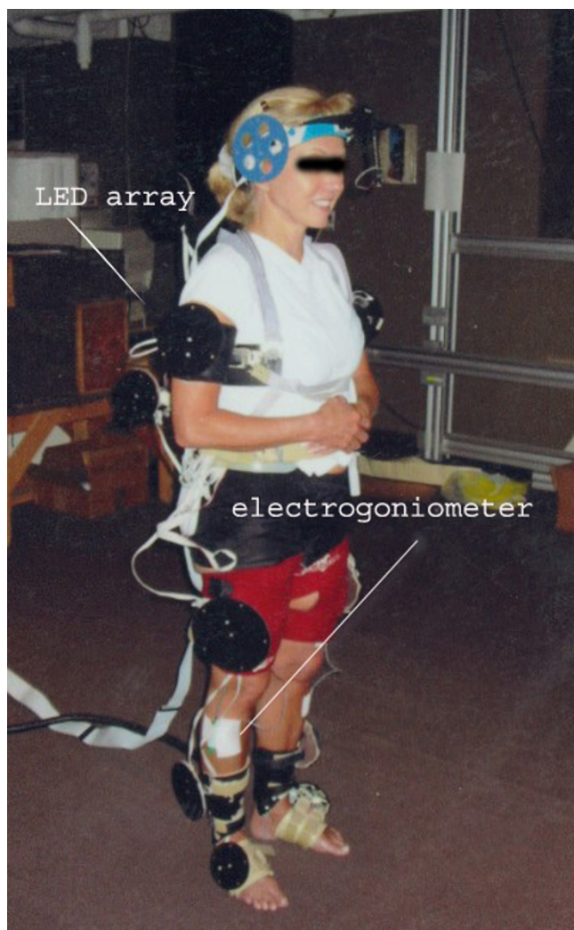
Figure 1 Photograph of a subject being tested in the MGH Biomotion Laboratory with both the IDEEA system and LED arrays in place.
