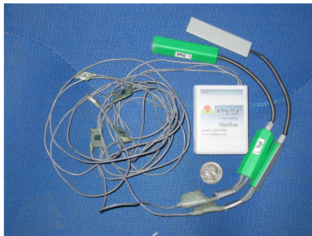
Figure 2 Photograph of the modified IDEEA system. The two electrogoniometers (green) were added to the system by MiniSun, LLC for our study.
