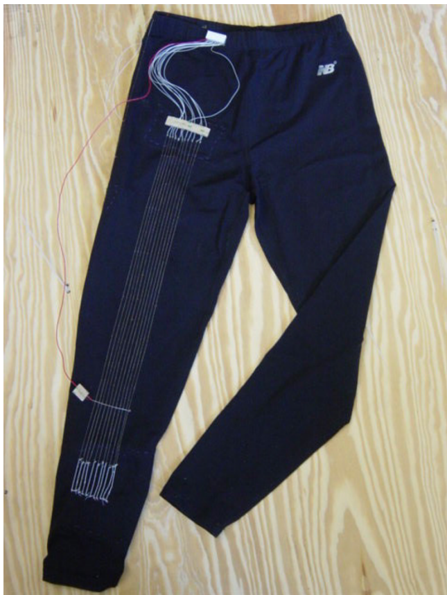
Figure 7 Prototype Sensing Garment. Spandex pants with conductive fiber sensors for lower body monitoring.
